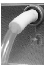
Fit the other piece of tubing into the external desufflation actuator
